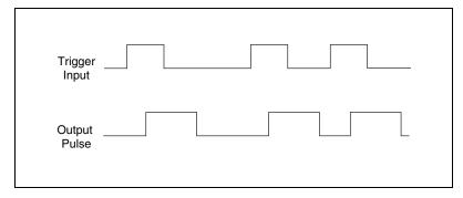
Figure 4-1. Output Pulse When Trigger Is Selected
